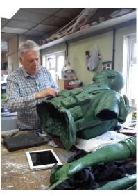
To turn the wax verisions of the sculpture into bronze the lost wax process was used for the parts of the bodies and sand casting for the base.
