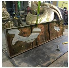
The separate parts were then welded together, the welds chased and the whole sculpture was sandblasted before being given the final finish, below.
